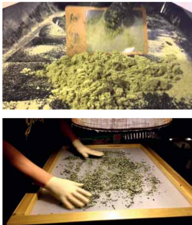
Figure 3.3 The production of cannabis resin through the 'sieving' method using a mesh screen
